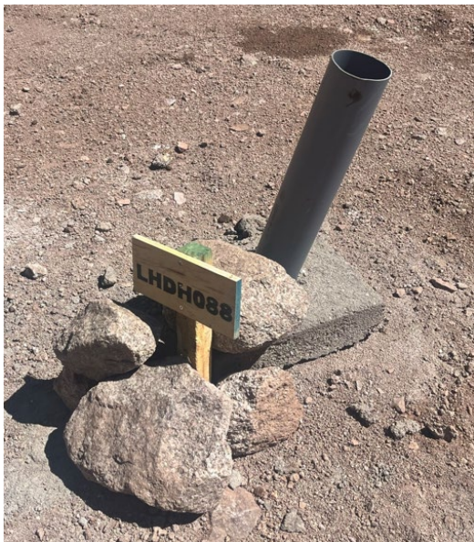
Figure 12-2: Los Helados LHDH088 Drill Hole Collar
